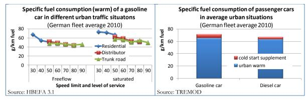
Figure 5: Specific final energy consumption of passenger cars in urban traffic situations
