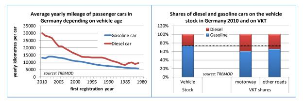
Figure 14: Relevance of vehicle age and engine type for the dynamic passenger car fleet composition in Germany
