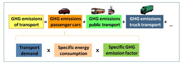
Figure 10: Calculation scheme for an urban transport GHG balance
