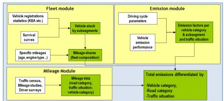
Figure 8: Emission calculation for road transport in TREMOD
