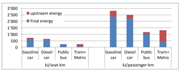
Figure 3: Energy consumption factors for different means of urban passenger transport
