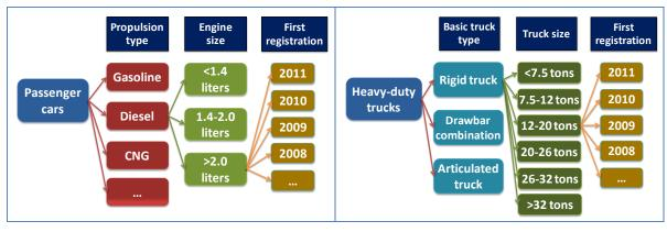
Figure 4: Fleet composition: Differentiation of road vehicle subsegments (exemplary)
