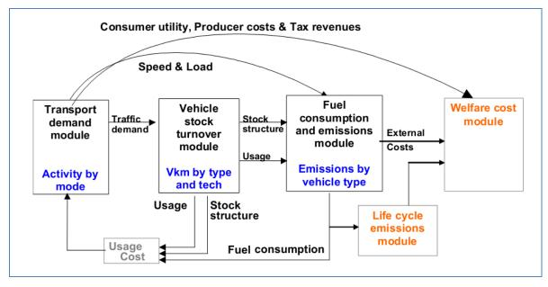
Figure 9: Model structure of TREMOVE
