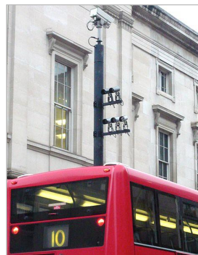
Picture 2: Cameras recording passing vehicles to enforce London's congestion charge (Photo: Wiki Commons)
