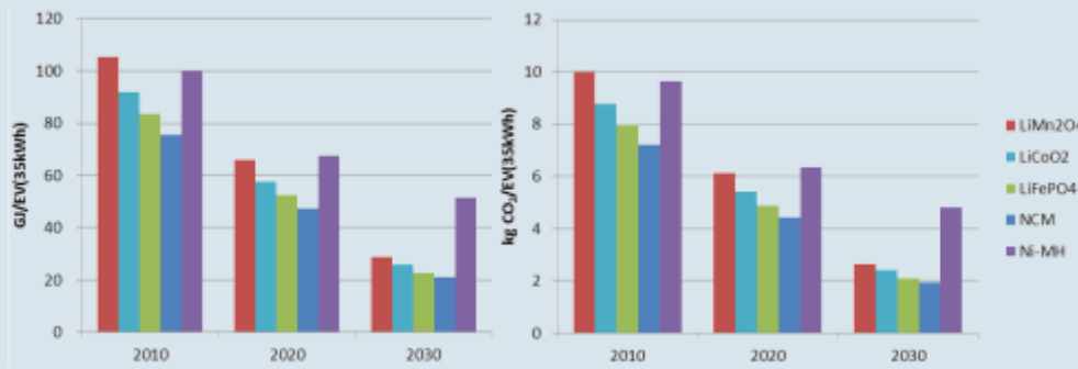
Figure 68: Vehicle-cycle a) energy use and b) CO 2 emissions of battery EV, 2010-2030
