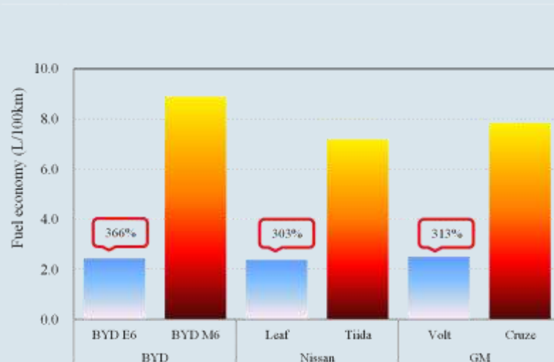
Figure 11: Comparisons of fuel economy between BEVs and the corresponding ICEVs, 2010
