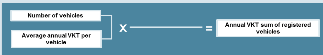
Figure 15: Calculation function for road transport activities in the basic approach (Source: IFEU 2014)
